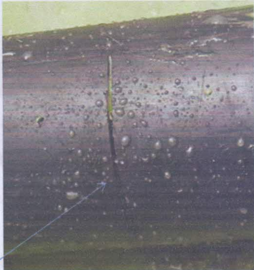
Point A, 150mm Hack saw cut on the cone (Before and after repair)
